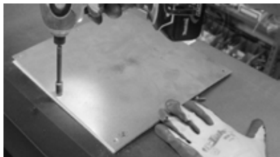
Step 1: Remove the eight (8) screws holding the top vent cover plate and gasket.
