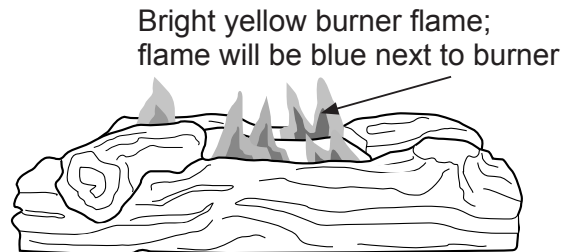
Figure 35 - Correct Burner Flame Pattern
