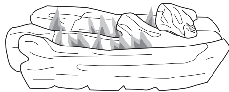
Figure 45 - Correct Burner Flame Pattern
