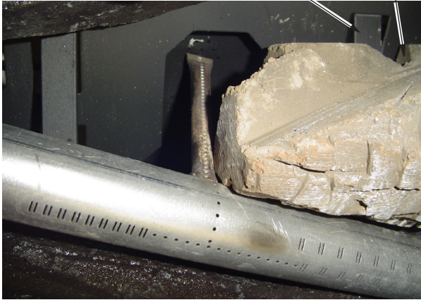
Figure 21B - Installing Charred Log Top Side View
