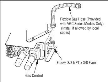
Figure 11 - Attaching Flexible Gas Hose to Heater Gas Regulator
