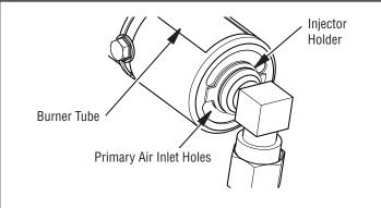
Figure 45 - Injector Holder On Outlet Burner Tube
