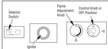
Figure 42 - Control Knob, Igniter Button and Remote Selector Switch
