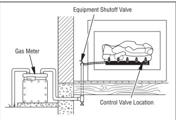
Figure 17 - Checking Gas Joints (Natural Gas Only)
