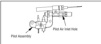
Figure 46 - Pilot Inlet Air Hole (Your pilot may vary from pilot shown)
