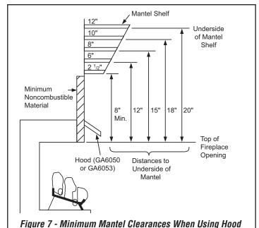
**IMPORTANT**: If you cannot meet these minimum clearances, you must operate heater with chimney flue damper open. Go to <u>Installing Damper Clamp Accessory for Vented Operation</u>, **page 10**.
