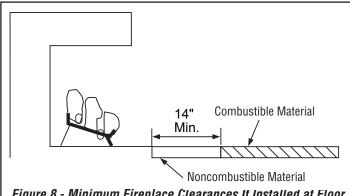
Figure 8 - Minimum Fireplace Clearances It Installed at Floor Level
